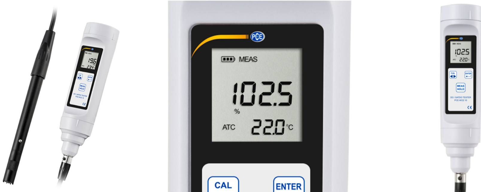
Oxygen meter PCE-WO2 10 waterproof oxygen meter with HOLD function / testing of oxygen content, oxygen saturation and sample temperature in water / battery operation / automatic temperature compensation
